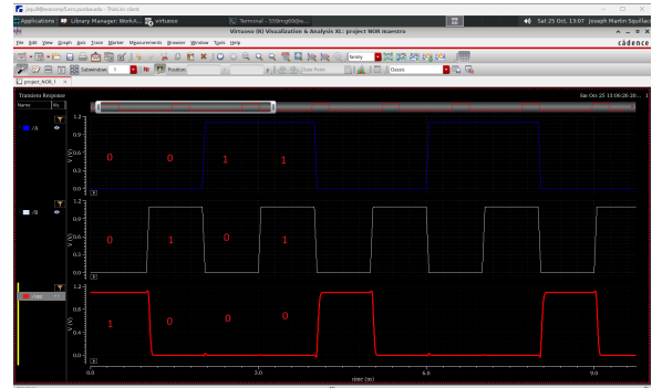
[19] Waveforms proving the NOR's functionality.
